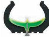
Ceramic fibers hold the puncturing object in place to prevent further tire damage.
