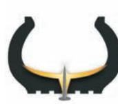
Ceramic bers hold the puncturing object in place to prevent further tire damage.
