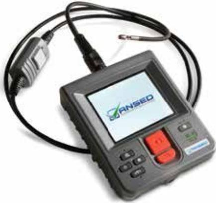
Versatile small diameter Video Scope Kit with unique 4.9mm diameter Switchable Dual Camera Probe. Change from front to side view with a click of a button.
