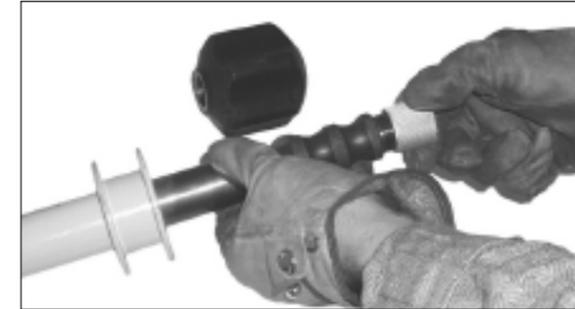
1. Users will often want to attach the optional 5 Pound Handle Weight to the Slide Sledge™ Multi-Head™ hammer to increase the driving force of the tool and to allow for a more comfortable hand position. To add the 5 Pound Handle Weight, start by removing the drive bar thread cap located on the drive bar.
