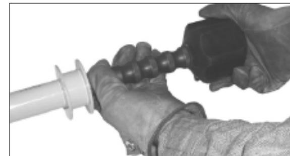
4. The 5 Pound Handle Weight is properly attached to the drive bar when it bottoms out on the main body of the drive bar. Be sure that the 5 Pound Handle Weight is seated fully prior to use.
