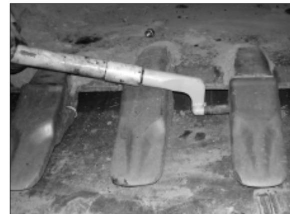
3. Place the pin into the pin placement cavity on the tip. Align the pin with the bucket tooth hole and bucket hole.
