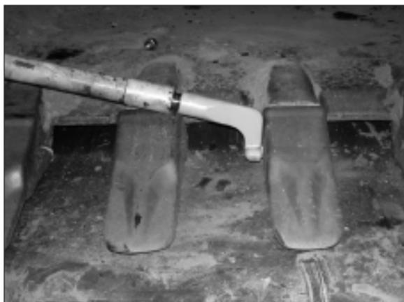
6. Drive the pin completely into position using the flat area located next to the pin placement cavity on the tip.
