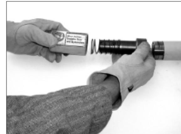
2. After removing the plunger housing, separate the plunger and plunger spring from the plunger housing. You can now replace any of the components. Reverse the procedure to install.
