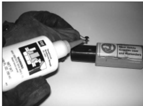
3. Prior to installing new retention clip, place a full circle of Loctite® 243 Threadlocker or CAT® Thread Lock Breakaway Strength 9S-3263 Threadlocker around screw. Place into plunger and secure.
