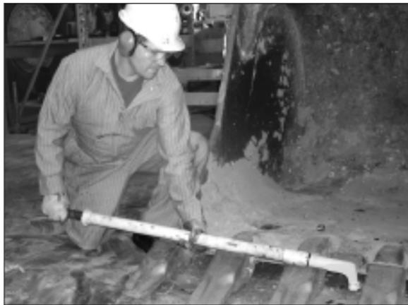
5. Thrust the drive bar forward to knock the pin in. Repeat until the bucket tooth pin inserter is almost flush with the bucket tooth.
