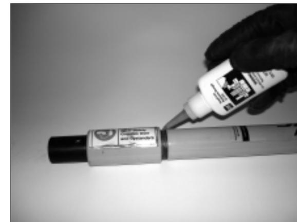
3. Before re-assembly, place a full circle of Loctite® 243 Threadlocker or CAT® Thread Lock Breakaway Strength 9S-3263 around the threaded area of the outer tube, then screw the plunger housing onto the threads on the drive bar tube in a clockwise direction. Be sure to thread plunger housing forcefully until the plunger housing can be threaded no further.
