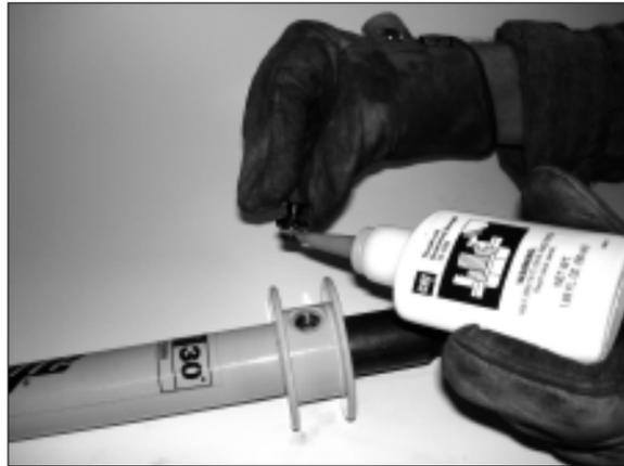
7. When the hand guard is secured, place a full circle of Loctite® 243 Threadlocker or CAT® Thread Lock Breakaway Strength 9S-3263 around the threaded area of the slide lock pin.
