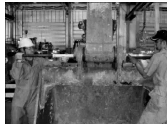
6. Before impacting the pin completely out of the cylinder, be sure to either a) have someone hold the pin, or...
