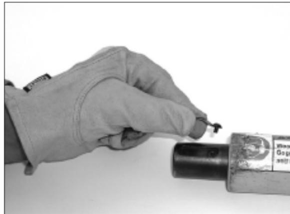
2. Remove the tip retention spring.
