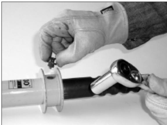
2. Remove the slide lock pin from the hand guard. You may now replace the slide lock or continue to remove the hand guard.
