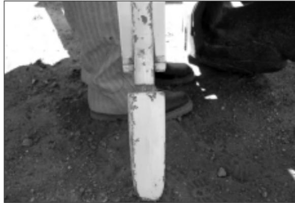
1. Attach the Scarifier Tooth Tip to the Slide Sledge™ Multi-Head™.
