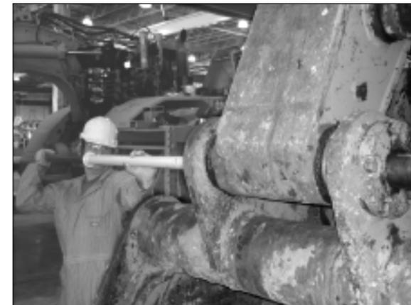
5. Continue to strike the pin until the pin is almost out of the cylinder.
