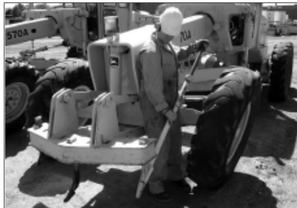
3. Draw the drive bar back and thrust the drive bar forward to separate the tooth from the arm. Repeat until the tooth is removed.
