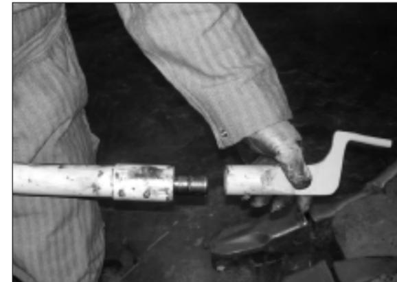
1. Align the tip's flat side with the flat side of the plunger. Slide the tip onto the plunger.
