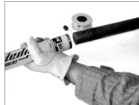
5. You may now slide out the drive bar to replace the drive bar retaining ring or repair / replace the drive bar.
