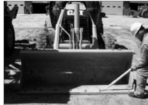
2. The Curved Chisel tip may be used to cut or shear metal bolts, pins and rivets up to 3/8" in diameter grade 8.
