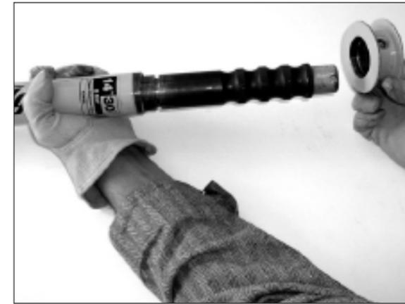
4. Slide the hand guard off the end of the drive bar.
