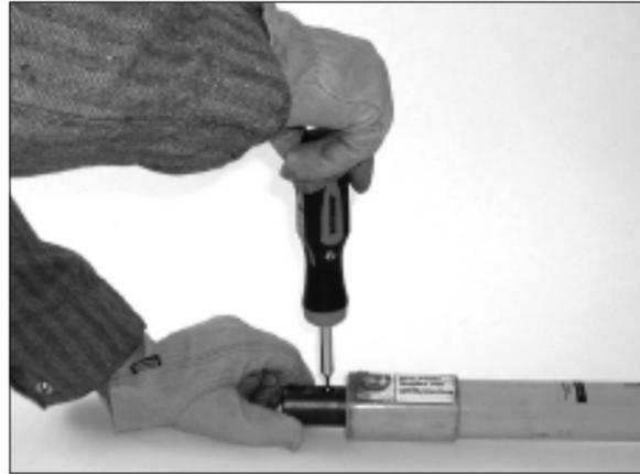
1. To remove the tip retention spring located on the plunger, heat the screw to 450 degrees Fahrenheit with flameless heat. Use a T-10 torque tip driver to remove the screw holding the clip in place.
