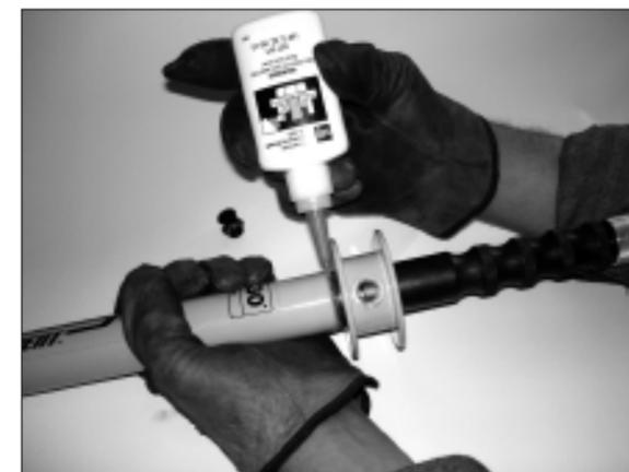
6. To reassemble, slide the drive bar with slide bar retaining ring back into the drive bar tube. Place a full circle of Loctite® 243 Threadlocker or CAT® Thread Lock Breakaway Strength 9S-3263 around the threaded area of the outer tube. Slide the hand guard over the drive bar end and thread the hand guard back onto the drive bar tube.
