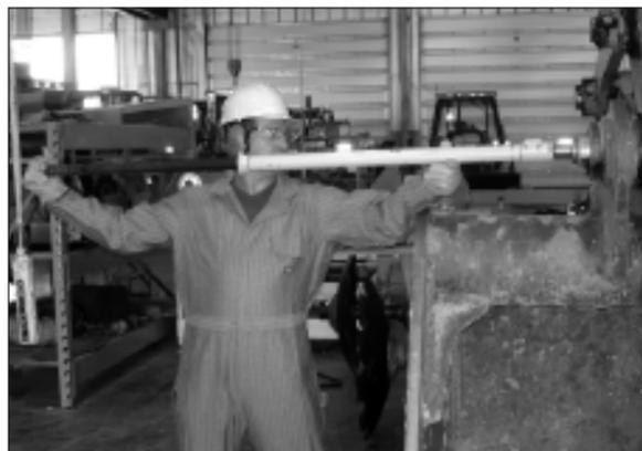
3. Press the tip against the pin to be removed and draw back on the slide bar.
