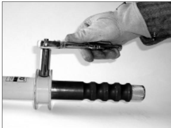
8. Use a 5/8", 12 point deep well socket to attach the slide lock to the hand guard. Tighten the slide lock pin until seated on the hand guard.
