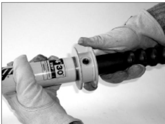
3. Prior to unscrewing the hand guard from the drive bar tube, heat the area to 450 degrees Fahrenheit to break down the Loctite® 243 Threadlocker or CAT® Thread Lock Breakaway Strength 9S-3263. Unscrew the hand guard by turning the hand guard in a counterclockwise direction.
