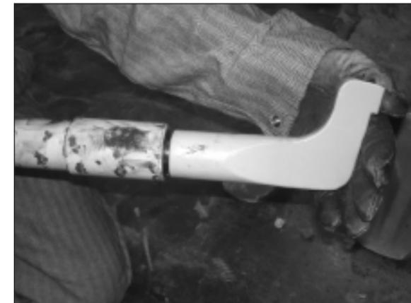
2. Slide tip onto plunger and press firmly until the tip cannot be inserted any further.
