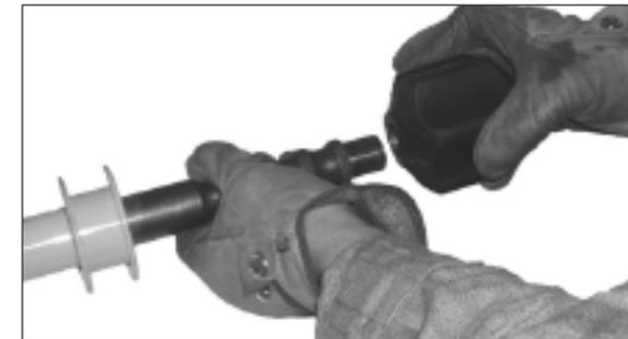
3. Take hold of the 5 Pound Handle Weight and align it with the threaded end of the drive bar. Hold the drive bar securely and start to thread the 5 Pound Handle Weight onto the drive bar in a clockwise motion.
