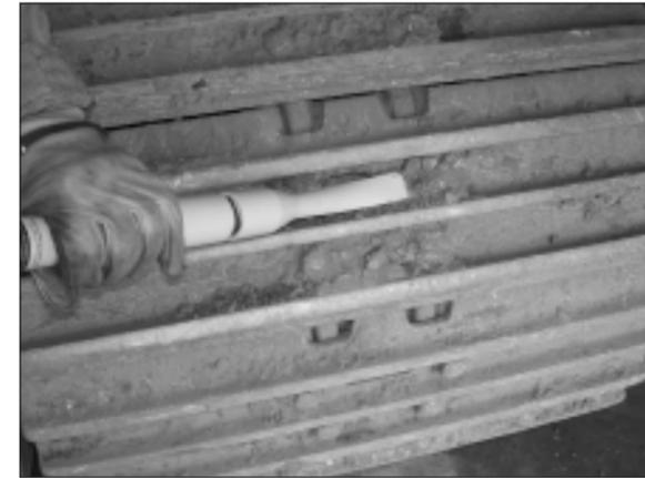
1. The Curved Chisel Tip is ideal for chopping away hardened debris to gain access to nuts, bolts and other vehicle components. Use the reach of the 46" tools to access tight areas.
